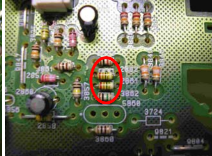
picture 3 Cut one leg of each of these 2 capacitors located near where the crystal was mounted – the two middle ones, numbered 2862 and 2861
