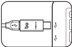
3. Many computers include more than one USB port. A second JitterBug filter can be used in parallel, but not in series with the first filter. Plugging a second JitterBug filter into an additional port will offer an incremental improvement to your system's overall sonic performance. That said, we do not recommend more than two JitterBug filters per computer.\*
