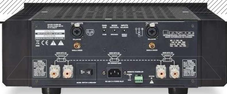
ABOVE: Single-ended (RCA) and balanced ins (combined XLR and 0.25in jack sockets) are joined by 1V and 2V input sensitivity options, a bridged output option, remote or local input switching and a single set of unswitched 4mm speaker binding posts
